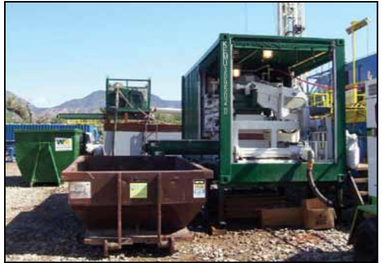
Figure 4 – KEMTRON's DFD System Can Eliminate the Need for Reserve Pits.
