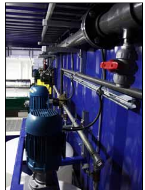
Figure 11 – KEMTRON's DFD Systems Incorporate In-Line Static Mixers and Sampling Port.
