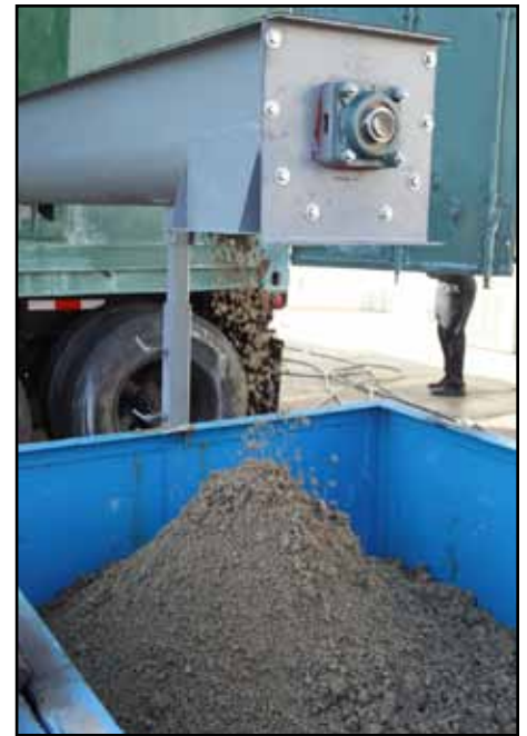
Figure 13 – Dry Solids Discharge from a KEMTRON DFD System
