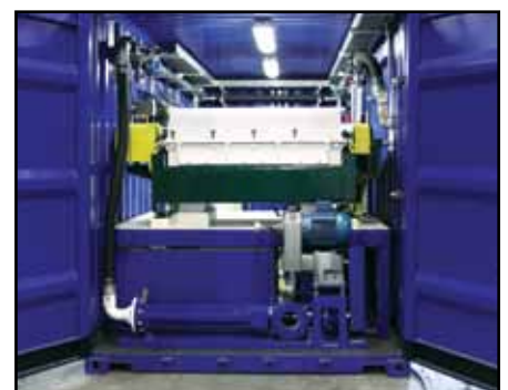
Figure 8 – 20’ DFD Systems Fed Via Progressive Cavity Pumps
