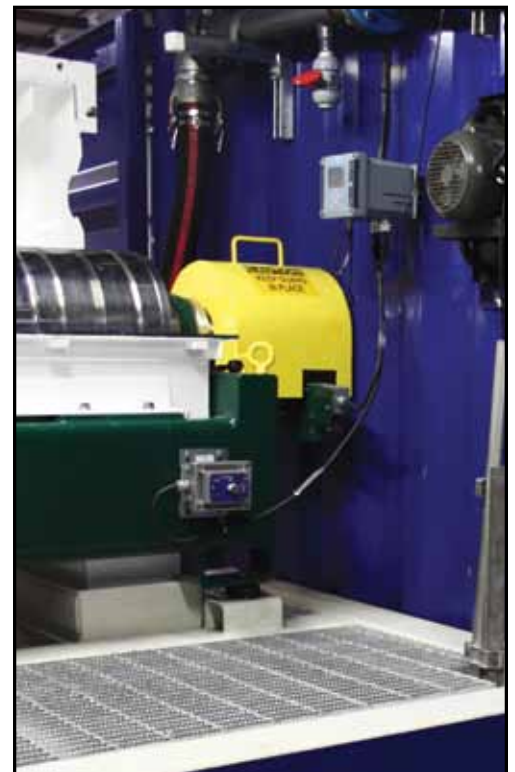
Figure 16– KEMTRON's DFD Systems Incorporating a HACH Turbidity Meter
