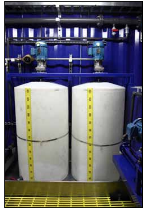
Figure 12 – KEMTRON's DFD Systems Incorporate In-Line Static Mixers and Sampling Port.
