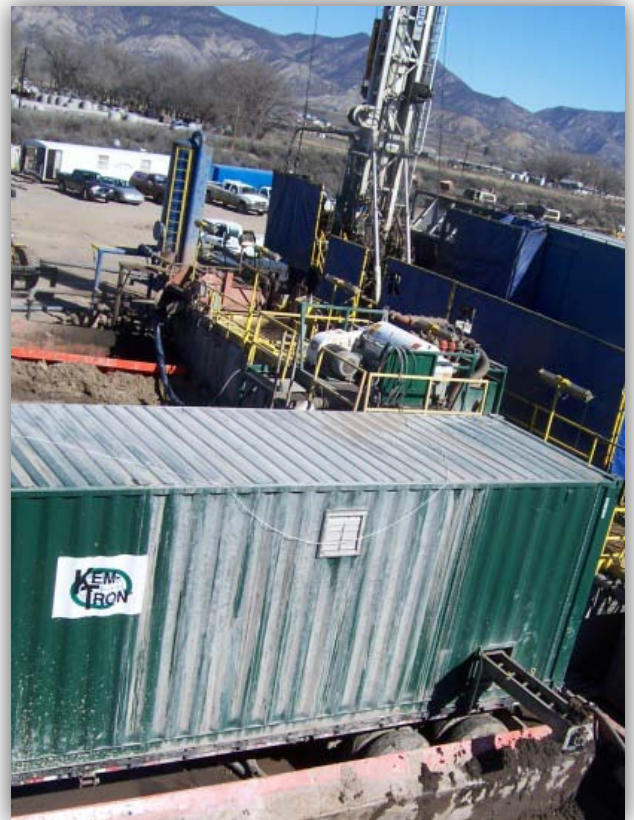
Figure 1 – Land-Based Drilling Fluid Management System Using KEM-TRON's KT-DW-40 Trailer-Mounted Dewatering System & KT-1448 Solids Control Centrifuges
